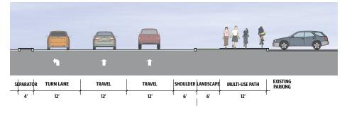
Medo Way. These combined elements allow for safer turning movements into businesses along the corridor without adding a lot of new roadway, making it a lower-cost option than Concept A.
