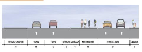
several frontage roads would be constructed on either side of the highway with designated points of access, along with three areas of back access road. Once on a frontage road, drivers are able to turn in and out of business parking lots at a slower speed, without having to pull directly onto the highway upon exiting.
